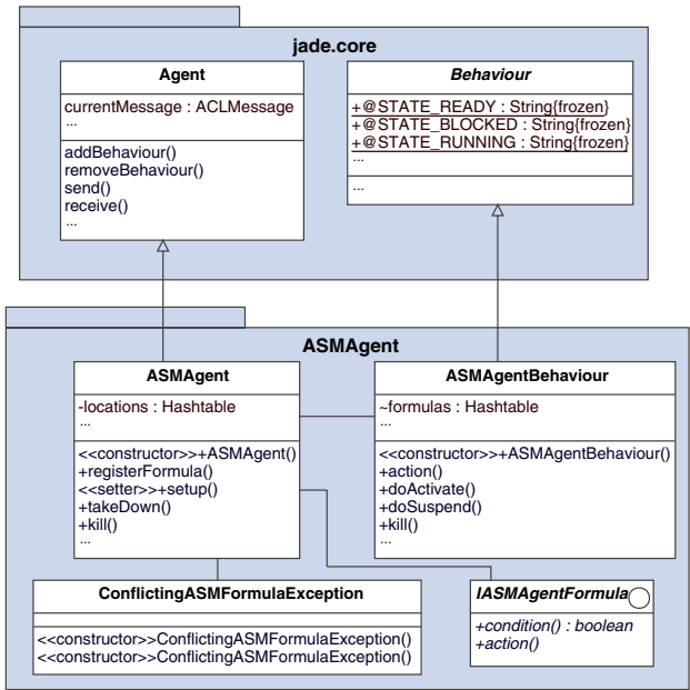
Fig. 2. UML diagram of the JADE implementation of ASM architecture
